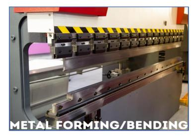
DMC's 10 CNC controlled press brake machines have up to 5-axis and rang up to 130-ton capacities.
