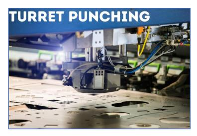
DMC has 4 turret press machines (3-22 ton, 1-30 ton), capable of punch diameters of up to 4.5", .020 to 3/16 thickness, and max table sizes of 50"x100" before repositioning.
