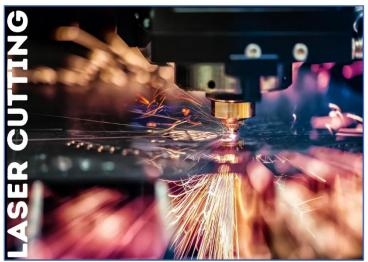
DMC's latest laser cutting technology has 9kW of power. We are cutting metals up to 1" in thickness mild steel and .5" aluminum and cutting tolerances as tight as .0002".
